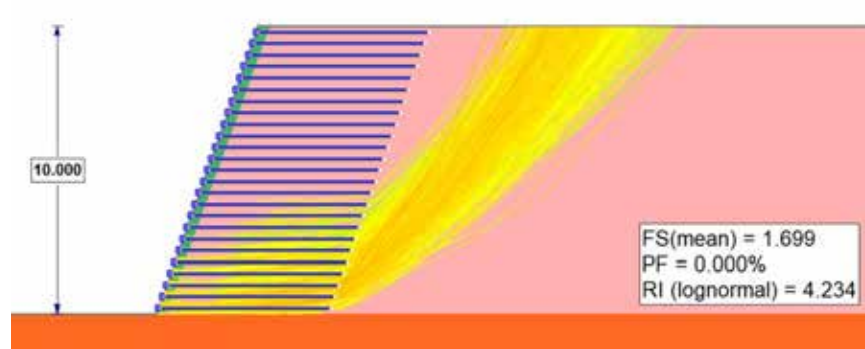
Figure 8. Failure surfaces with anisotropic SCL (not correlated, r = 0,6 )
