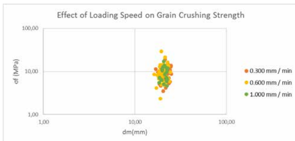
Figure 7. Effect of Loading Speed on Grain Crushing Strength
