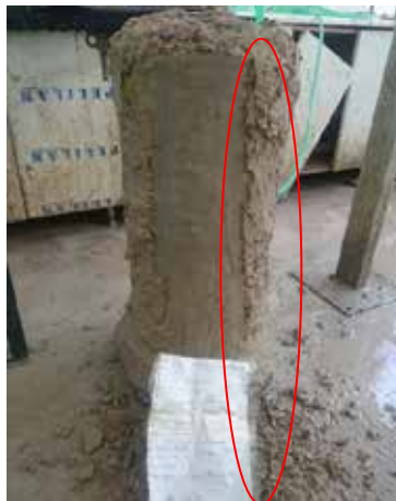
Figure 4. An interface layer (stiff clay) between column surface and untreated soil
