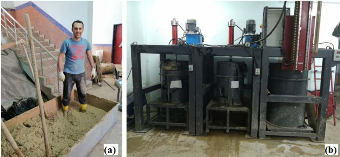
Figure 3. a) Mixing the soil in target water content, b) consolidation stage of the soil under hydraulic piston
