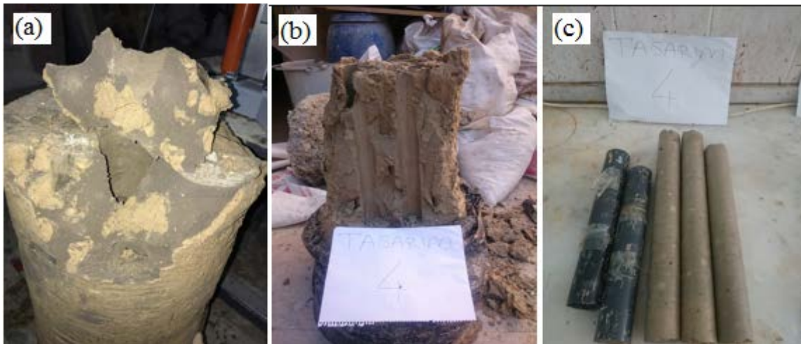
Figure 6. a) Nonhomogeneous mixing soil-cement (RS<60 rpm), images from Design 4 b) inside of DMC and c) core samples (homogeneously mixed DMC, RS=60 rpm)
