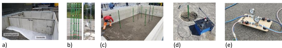
Figure 1. a) The reinforced concrete basin, b) Types of tubes, c) Filling of sand in layers, d) Injection with double packer, e) Measurement setup
