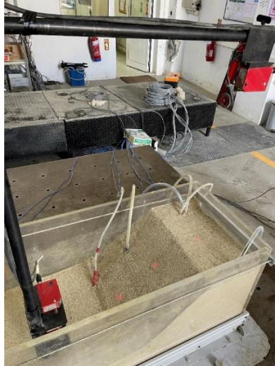
Figure 1. Test set-up of the embankment models.
